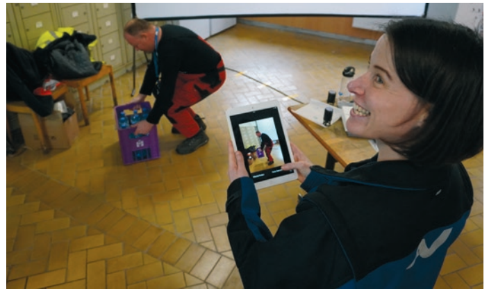
Posture scores for correct lifting and carrying: A case of mineral water and special analysis software reveal common posture errors.
