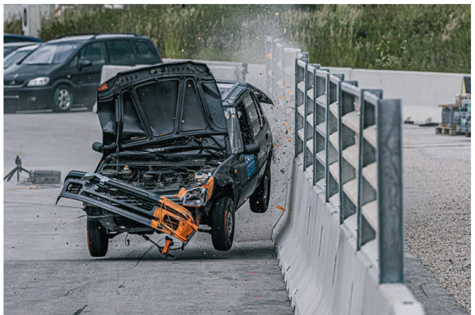
Impact testing for Pass&Safe®: The moment of truth at the test site in Allhaming shows that the safety for workers behind the impact, visual and splash protection exists on paper, but also can be tested and documented in practice.
