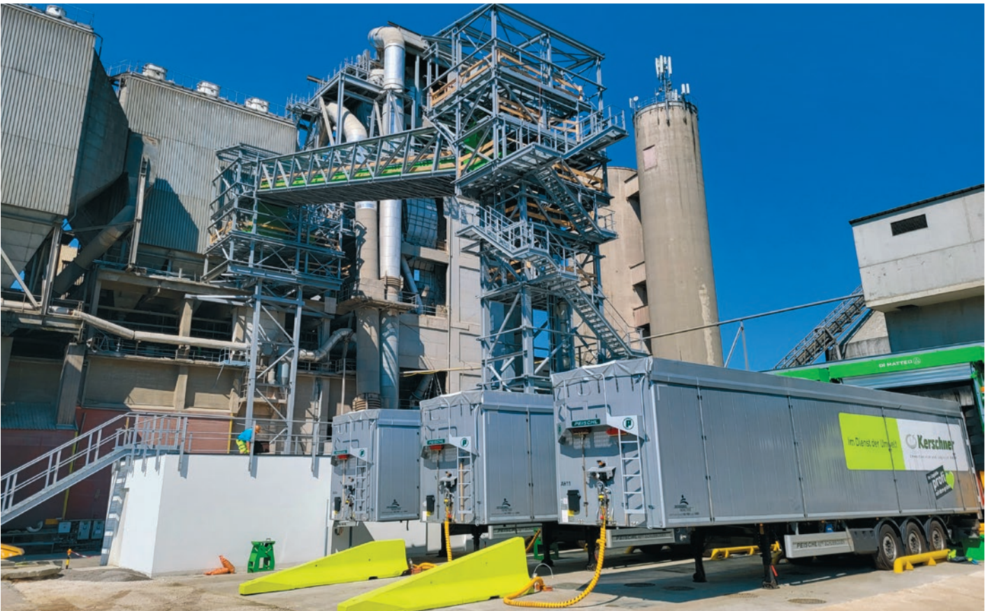
Kiln-ready delivery: In the new EBS 5 loading terminal, SRP deliveries go directly from the Kerschner Umweltservice trailer onto the conveyor.
