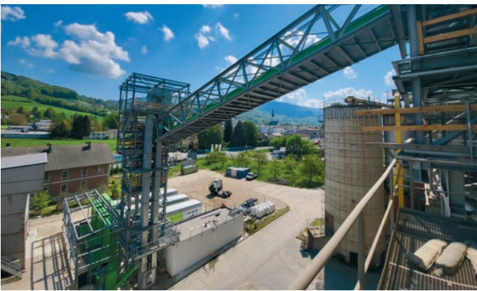
Alternative fuel supply around the clock: Fuel is fed into the calciner's refractory piping via a trough chain conveyor.
