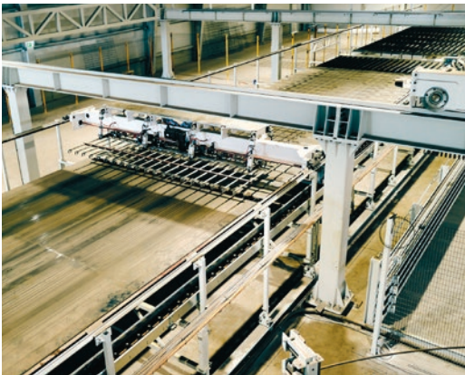
Up to 200 square metres of reinforcement mesh per hour can be welded in variable sizes.
