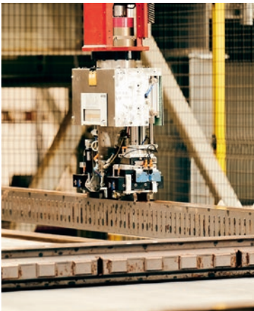
Left: The demoulding and shuttering robot identifies the shutterings with a camera and a laser scanner. Right: Post-processing station and curing chamber.
